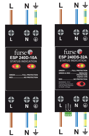
Figure 2a & 2b: Installation of 'D' and 'DS' variants.
