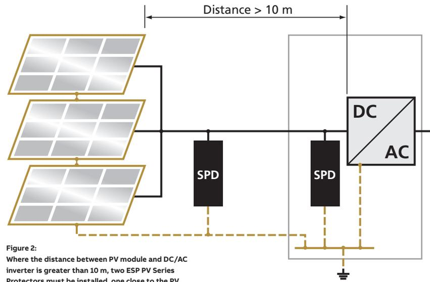
**Figure 2:** Where the distance between PV module and DC/AC inverter is greater than 10 m, two ESP PV Series Protectors must be installed, one close to the PV module and the other close to the DC/AC inverter.
