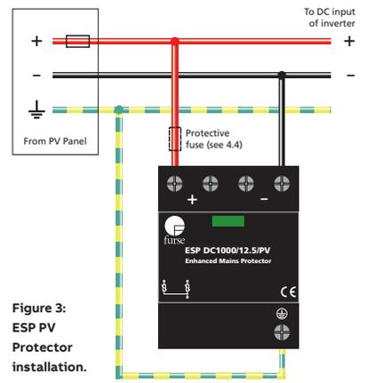
**Figure 3:** ESP PV Protector installation.
