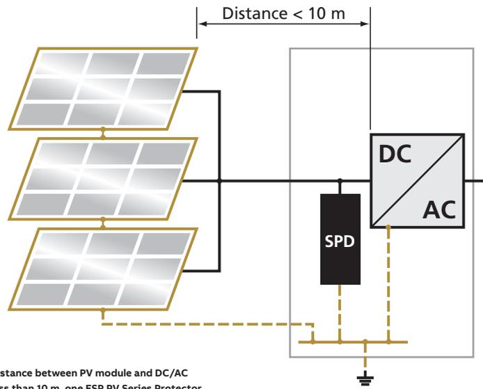
**Figure 1:** Where the distance between PV module and DC/AC inverter is less than 10 m, one ESP PV Series Protector suffices, installed close to the DC/AC inverter.
