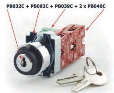
3-Way Key Switch + Coupler + 1 x NO Contact + 2 x NC Contacts PB032C + PB093C + PB039C + 2 x PB040C
