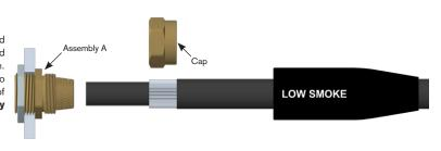
2. Slide the Cap along the cable and splay armour wires to match Assembly A Cone.
