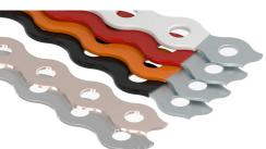
Multi-Purpose Fixing Band is a versatile product used in many applications. It is available in three widths 12, 17 & 26mm manufactured from Carbon Steel coated as standard used to secure cables, pipes, ducts & conduits. Available bare galvanised (G) or coated in Black (B), White (W), Red (R) and Orange (O). Other materials offered are Copper and Stainless Steel.
