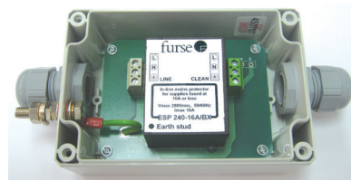
Figure 8: The ready-boxed ESP 240-16A/BX (or ESP 240-5A/BX, ESP 120-5A/BX, ESP 120-16A/BX, ESP 277-5A/BX or ESP 277-16A/BX) can be flat mounted via M5 mounting holes located outside the inner seal of the unit.
