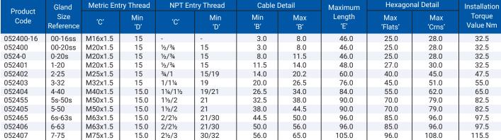
All dimensions except NPT are in mm. Intermediate thread sizes are available on request. NPT threads should be tightened "wrench tight".
