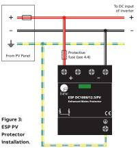
Maximum torque is 4.5 Nm power terminals, with cable stripping length 11 mm. The torque rating for the volt-free contacts is 0.25 Nm and cable stripping length 7 mm.
